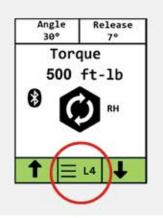
To switch the tool to a lower level select Admin > Access Level. Scroll to the level desired and press the center button to select. The new Access Level is now displayed in the center box at the bottom of the screen. A password is not required to switch from a higher level to a lower level.
