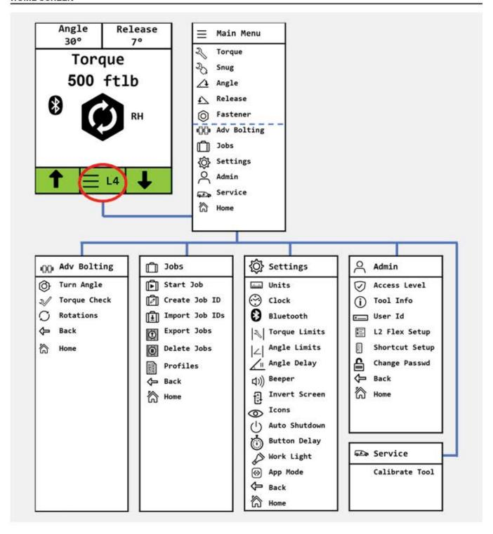
This guide provides instructions for operating the tool using the menu system and functions shown on this page. This menu structure allows users to quickly access bolting functions starting with the Home Screen and working through the main menu and sub-menus.
