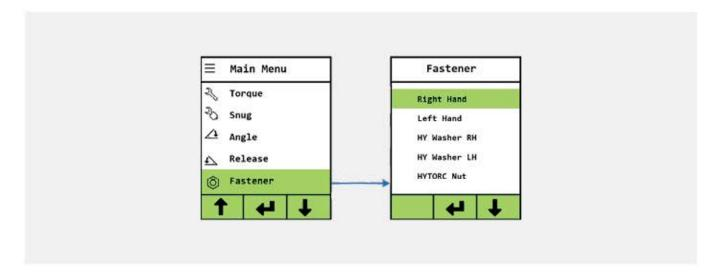
For traditional RH or LH fasteners, the tool assumes use of reaction arms and displays a safety message, "Press any button to start operation," to keep the user's hands away from any pinch point. For the HYTORC Washer (HWR, HWL) and the HYTORC Nut (HN) a reaction arm is not required and the safety message is not displayed.
